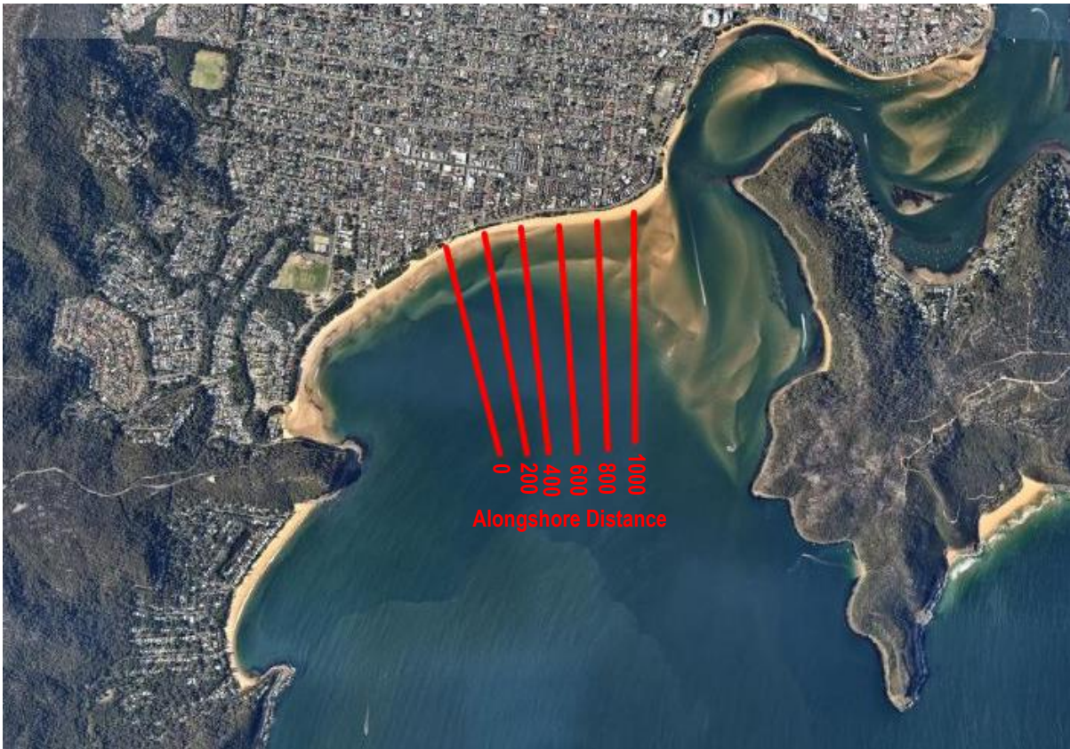
Figure 5: Location of profile transects used for SWAN model data extraction
