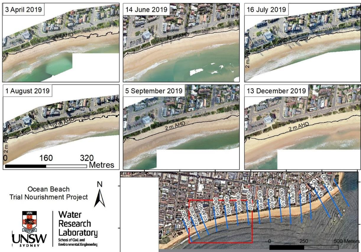
Figure 8: Movement of the 2 m AHD contour within nourishment bund during monitoring period
