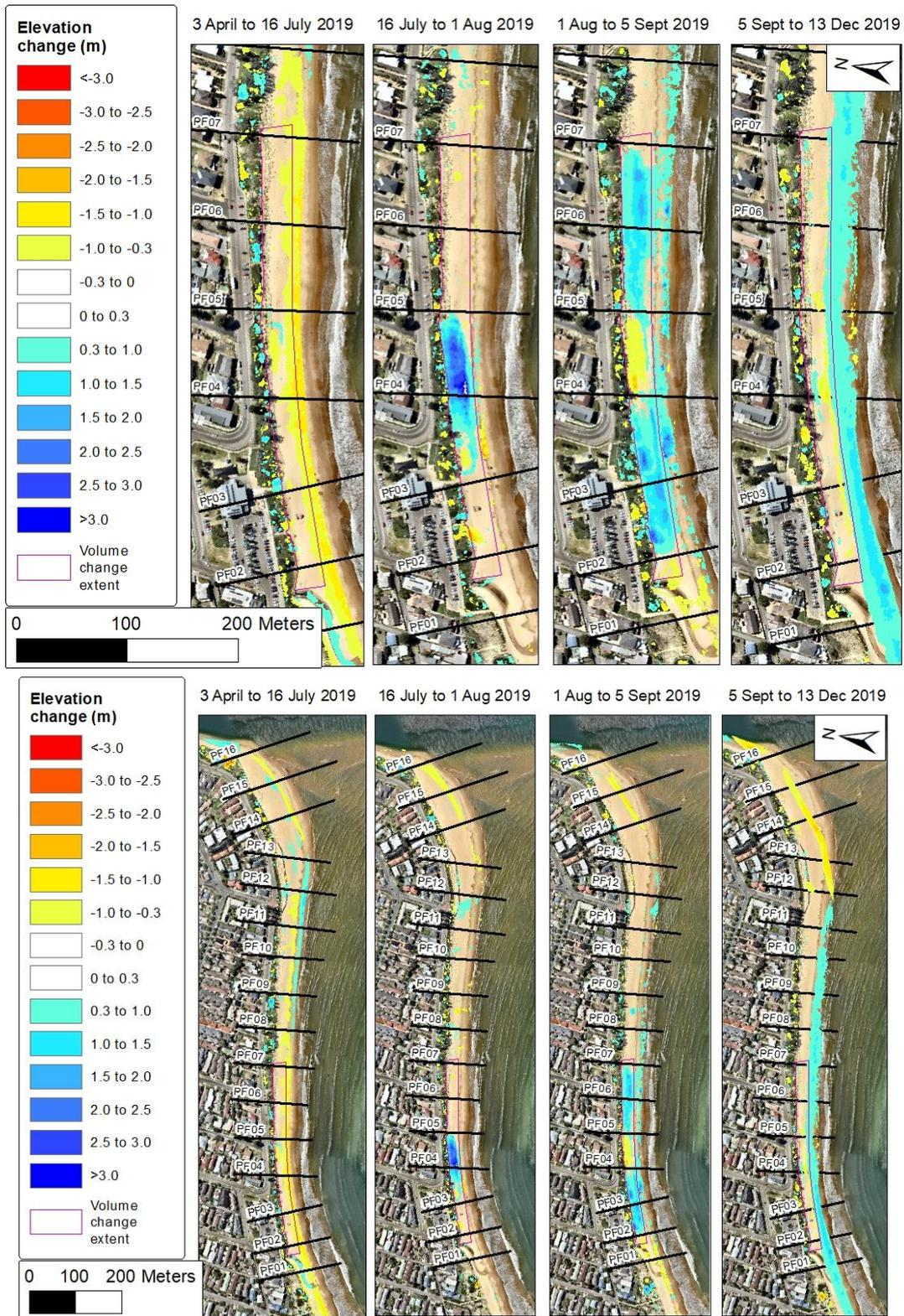
**Figure 7: Vertical elevation changes throughout monitoring within the nourishment placement zone (top) and for Ocean Beach to Ettalong Point (bottom)**
