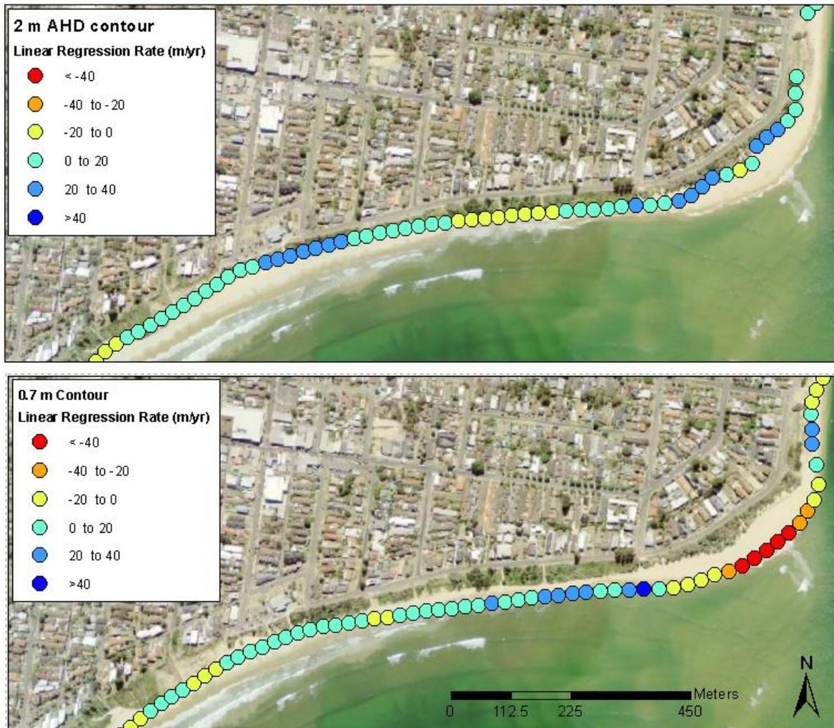
**Figure 9: Analysis of the linear regression rate of movement between April and Dec 2019 of the 2 m AHD contour (top) and the 0.7 m AHD contour (bottom)**
