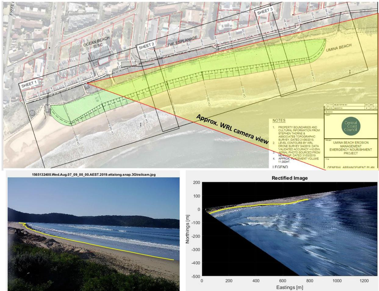
**Figure 2: Camera field of view (top), oblique camera view and digitised shoreline (bottom left); rectified image showing shoreline and wave breaking on ebb tide shoal (bottom right)**
