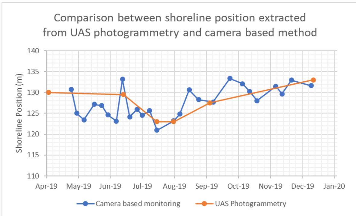
**Figure 11: Comparison between camera derived MSL shorelines and measured survey data**
