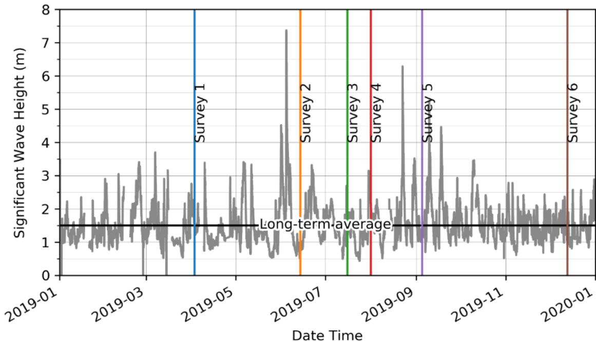
**Figure 4: Offshore significant wave height recorded at Sydney wave buoy (MHL, 2020)**
